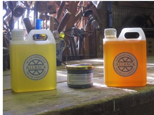
Linseed oil soap, a 7-oz sample of linseed oil paint, and purified raw linseed oil
